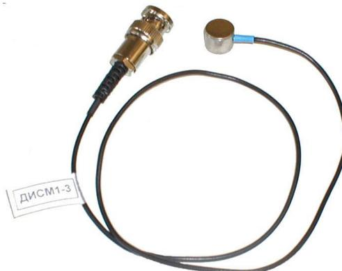
Fig. 2. Exterior view the AE sensor
